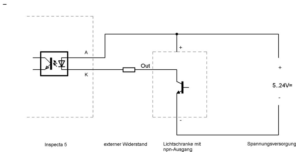
OK1 is the optocoupler on Inspecta-5; R1 and the transistor (e.g.: the light barrier containing this transistor enthält) are external components.
