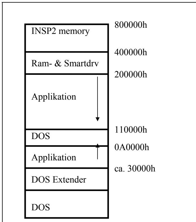
This is an example for 4MB main memory and 2\*2MB INSP2 memory. There is also 1MB SMARTDRV and 1MB RAMDRIVE installed.
