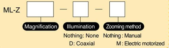
High-resolution super low magnification motor zoom lens
