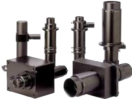
MML Zoom Lenses are high-performance lenses with integrated coaxial episcopic illumination designed based on telecentric optics. Multiple zooming, long working distance, and an integrated coaxial episcopic illumination system that covers the entire view allow for recognition of all types of objects. Manual type products and electric zoom type ones with a stepping motor are available.
