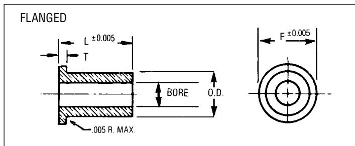
**Material:** Heavy Duty TFE Filled Polymer
