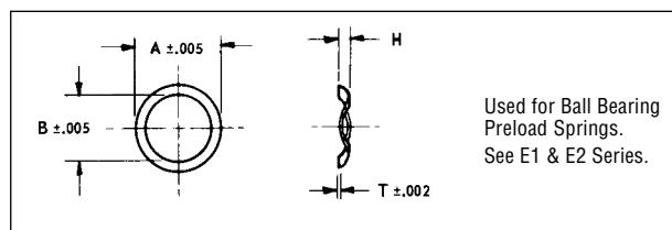
**Material:** 300 Series Stainless Steel - spring tempered, except where noted with " \* " it is high carbon steel ASTM-A684
